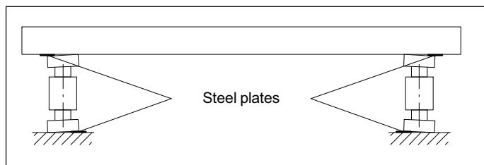
Structurally, this effect can be counteracted by shifting the bearing points on the weighbridge as far upward as possible, towards the neutral bending axis.
