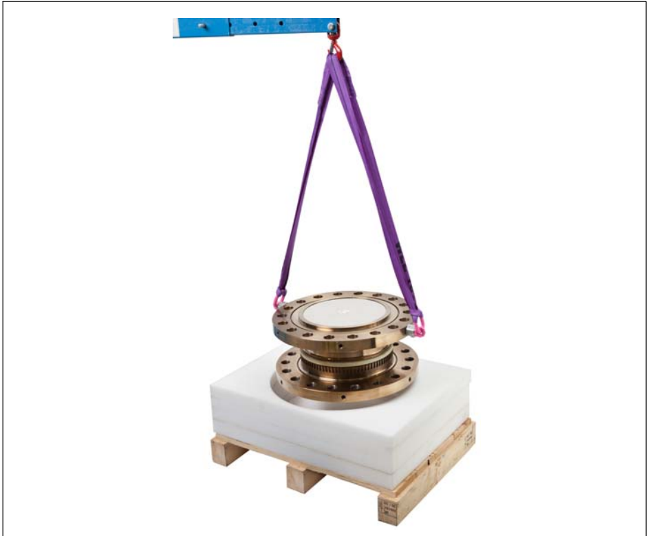
Fig. 5.2 Hoisting the rotor out of its packaging
