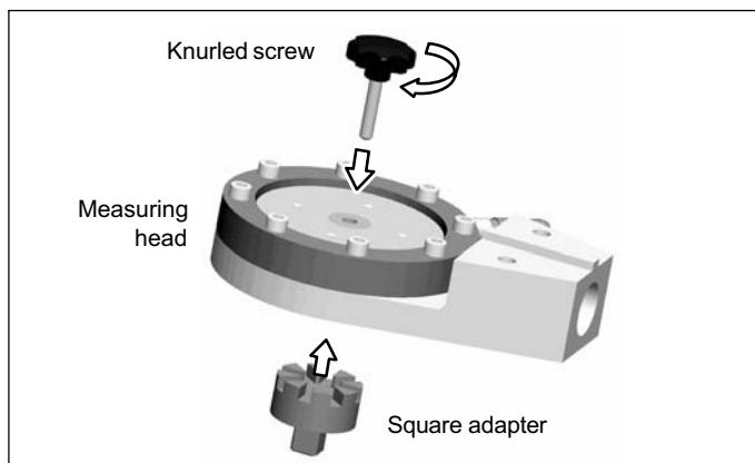
Fig. 5.2 Fitting the square adapter on the measuring head
