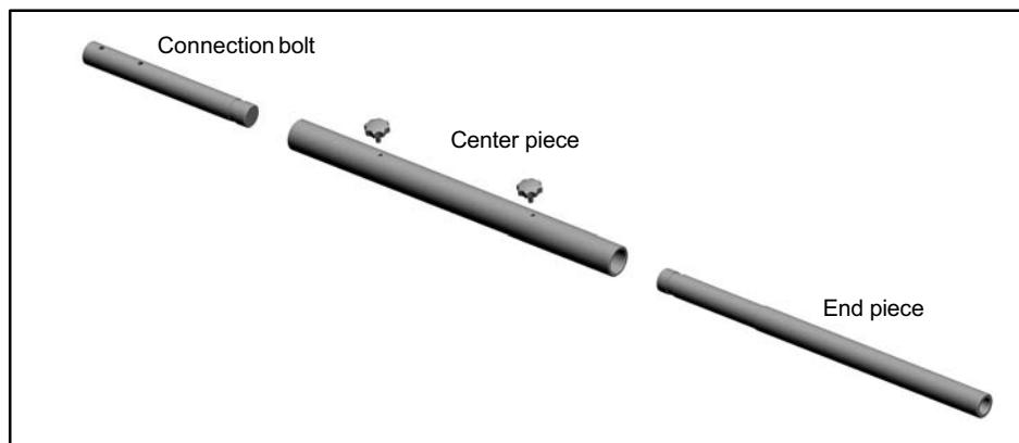
Fig. 5.5 Three-piece lever (500 N·m, 1 kN·m)
