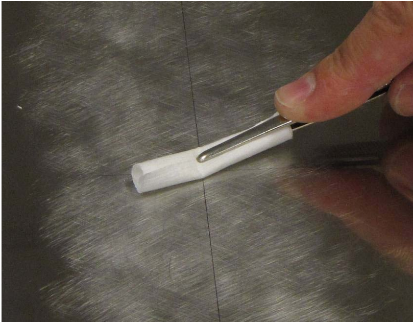
Fig. 2.2: Final cleaning of the installation point
