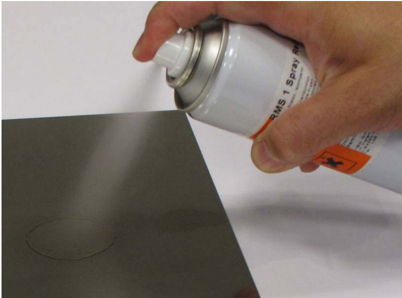
Fig. 1.1: Spraying the measuring point with 1-RMS-SPRAY
