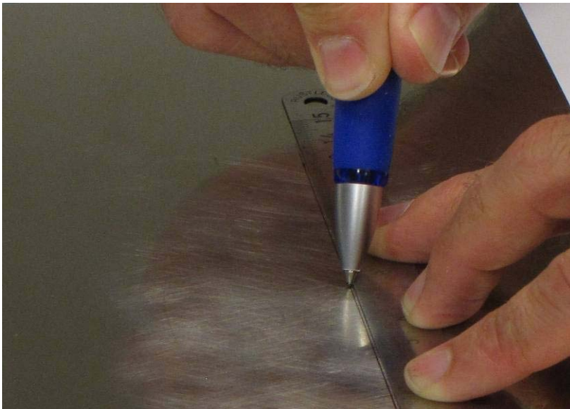
Fig. 2.1 Marking the marking lines
