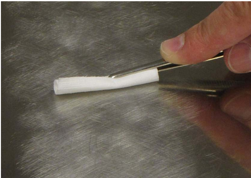
Fig. 1.4: Cleaning the roughened installation surface
