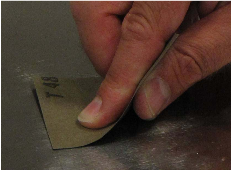
Fig. 1.3: Roughening the surface of the measuring body
