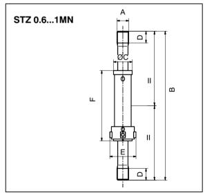
These special KD and STZ transducers are used to check out material testing machines and are designed in accordance to ISO 376. They are compressive force transducers and tensile force transducers that, because of their maximum overall height, are suitable for checking material testing machines according to ISO 7500-1.
